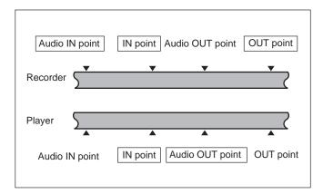
You can set audio cut in, crossfade, fade in, and fade out effects, including their durations, by menu selection. For details, refer to the Installation Manual.
