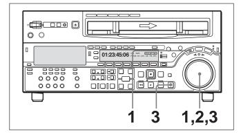
**1** Press the SHUTTLE button or search dial so that the SHUTTLE button is lit.
