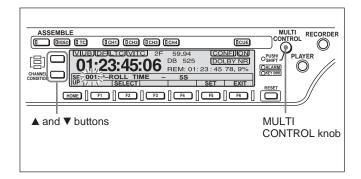
When the menu item number displayed in the menu display is flashing, you can change the menu item by turning the MULTI CONTROL knob.
