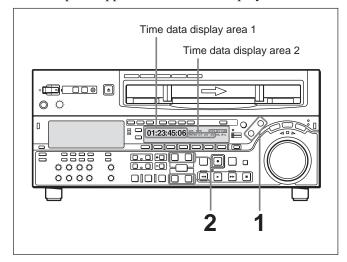
Press the RECORDER button or PLAYER button to select the VTR on which you wish to check the edit point.
