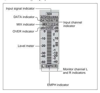
**Input signal indicator:** Indicates the currently selected input signal ('SDI', 'AES/EBU', 'ANA' for analog) for the corresponding audio input channel.
