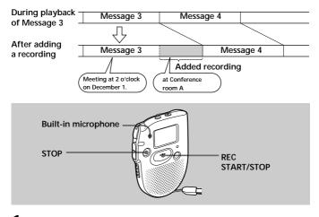
1 During playback, press REC START/STOP for more than 1 second. The OPR indicator lights in red and "R-PLUS" flashes three times. Speak into the built-in microphone. The display will then change to the remaining recording time.
