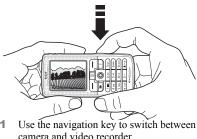
Press the camera button halfway down to automatically focus. When the green dot stops flashing, press all the way down to take a picture or start recording. If the green dot flashes slowly, the picture is not in focus and you may have to try again.
