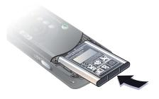
3 Insert the battery with the label side up and the connectors facing each other.
