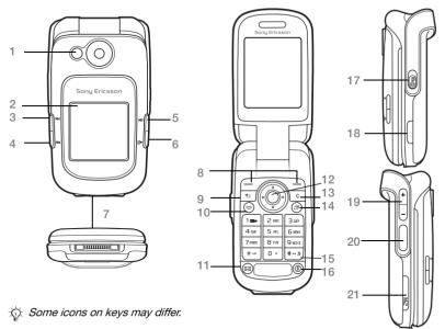
1 Camera lens 2 Screen 3 Forward/next button 4 [44] Rewind/previous button 5 Play/stop button 6 **[** Menu/togale button 7 Connector for charger, handsfree and USB cable Selection kevs 8 9 Back Kev (+) 10 ( Internet Kev 11 Messaging key 12 Navigation key 13  $\overline{C}$ Clear kev (P) Activity menu key 14 (#\_#) Silent key 15 16 **(I)** Power on/off button 17 Keylock switch (-)1/-18 Infrared port 19 Volume keys, camera zoom (1 +)20 Camera Button
