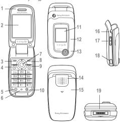
Ear speaker Screen 3.8 Left and Right Selection Keys Back Kev (<del>-</del> (X) MEdia Net Kev Microphone 0 Navigation Key 9 Clear Key (c) 10 Power On/Off 11 External Display 12 Front Style-Up<sup>TM</sup> Cover 13 Camera 14 Loudspeaker 15 Back Style-Up<sup>TM</sup> Cover 16 Push to Talk (PTT) Key 17 Volume 18 Infrared Port
