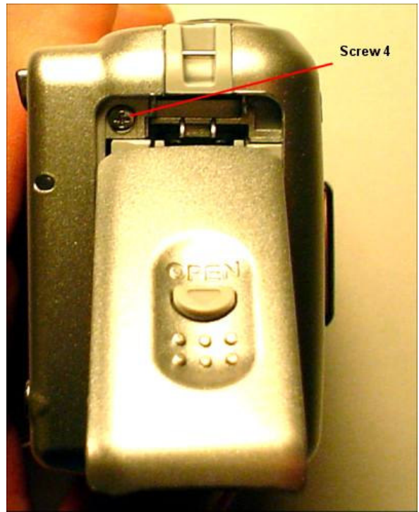
Remove screw 4 from under the battery door.
