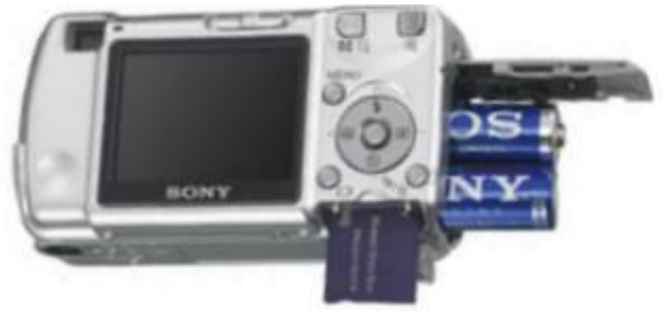
Remove the 2 AA batteries and Media Card
