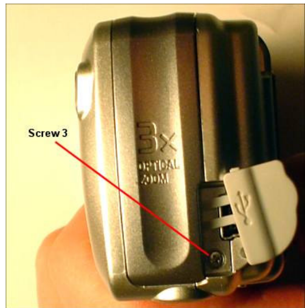
Remove screw 3 from under the USB connector door.
