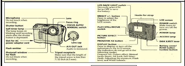
The Mavica MVC-FD83 is a digital still camera that can record both digital still as well as moving images. It uses a MS-DOS floppy disk as a medium for recording images. The disk can be formatted either using the camera or a PC.
