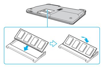
If you use only one memory module, make sure to insert it to the slot that is closer to the back of your computer.
