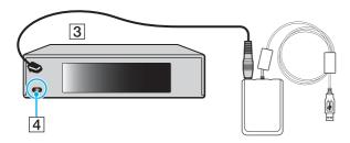
Do not cover the infrared port when attaching the remote sensor control.
