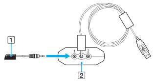
2 Remove the adhesive tape cover from the bottom of the remote sensor control (1).
