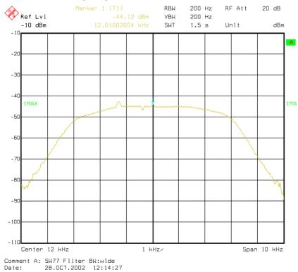
The recommended replacement filter is a Murata CFWM455GY, which has the same footprint as the original filter, but a bandwidth of appr. +/- 4,5 kHz. The bandwidth is shown in following diagram:
