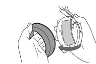
Hang the edge of the ear pad on one side of the ear pad around the driver unit as illustrated
