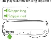
When you press and hold the jog lever until the voice guidance of "Zappin long" is heard, the playback time of song clips changes to about 15 seconds (Long). When you press and hold the jog lever until "Zappin short" is heard during "Long" playback, the playback time of song clips returns to about 4 seconds (Short).
