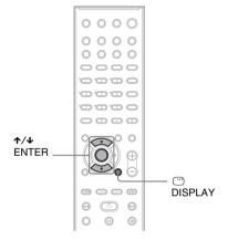
1 Press © DISPLAY when the system is in stop mode.
