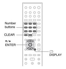
Press DISPLAY. (When playing a DATA CD with JPEG image files, press DISPLAY twice.)
