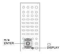
Press © DISPLAY when the system is in stop mode.
