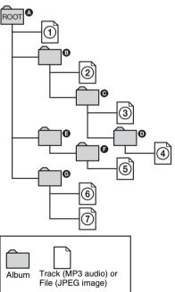
When you insert a DATA CD and press ▷, the numbered tracks (or files) are played sequentially, from ① through ②. Any subalbums/tracks (or files) contained within a
