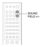
Press SOUND FIELD +/- on the remote repeatedly until "A.F.D. AUTO" appears in the front panel display.
