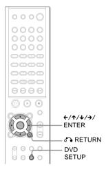
In stop mode, press DVD SETUP. The Setup Display appears.
