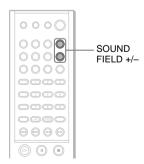
Press SOUND FIELD +/- on the remote repeatedly until "C.ST.EX A (or B, C)" appears on the front panel display.
