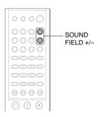
Press SOUND FIELD +/- on the remote repeatedly until the sound field you want appears in the front panel display.
