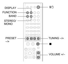
Press FUNCTION repeatedly until FM or AM appears in the front panel display.
