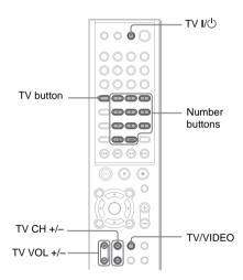
Press and hold TV I/ $\bigcirc$  while entering your TV's manufacturer's code (see the table) using the number buttons. Then release TV I/ $\bigcirc$ .
