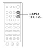
Press SOUND FIELD +/- on the remote repeatedly until "2CH STEREO" appears in the front panel display.
