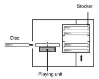
The disc changer consists of a playing unit and a stocker which transports the discs to the disc slot and the playing unit.
