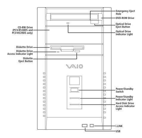
A For your convenience, your computer includes USB and i.LINK connectors on both the front and back panels, allowing you to connect to either set of connectors. The i.LINK connector on the front of your system is a 4-pin connector.
