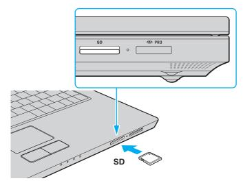
3 Carefully slide the memory card into the slot until it clicks into place. Do not force the card into the slot.
