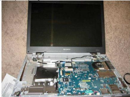
15. Remove the two black screws that are holding the HDD case to the motherboard.
