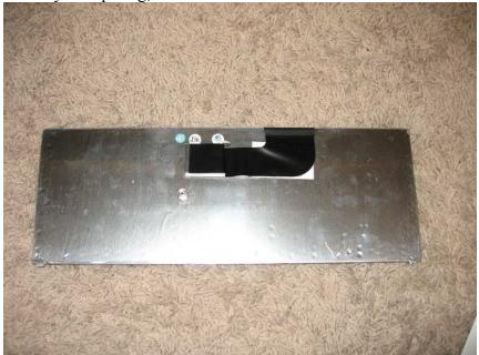
12. Remove the screw underneath the keyboard. Note the size of the screw. This screw is longer than the other screws.
