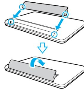
Unlock the battery's **LOCK** switch before installing the battery, and then lock the switch after installing.
