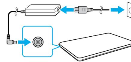
With the battery pack installed on your computer, plug the power cord and the AC adapter into an AC outlet and the computer.
