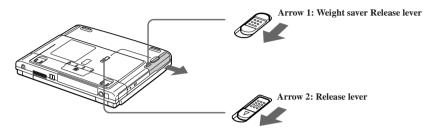
2 After removing the weight saver, pull out the weight saver's hinged arm and fold it into the weight saver.
