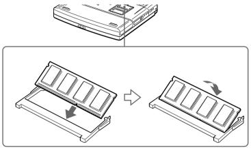
1 Slide the memory module into the slot. 2 Press the module into place until it clicks.
