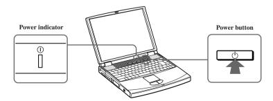
A If you hold the power button in the On position for more than four seconds, the computer turns off.
