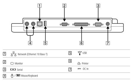
The port replicator can be powered only with an AC power adapter. Do not remove the AC adapter from the port replicator or the AC outlet while using the port replicator; this may cause data damage or hardware malfunctions.
