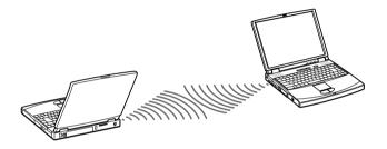
A Infrared communication capability can be turned on and off. By default, it is disabled when your system is shipped. Use the infrared icon in the Windows Control Panel to enable/disable infrared communication.
