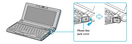
2 Plug one end of the phone cable into the jack on the inside of the phone line jack cover. Make sure you insert the phone cable from the rear of the computer and that the modular jack clicks into place.
