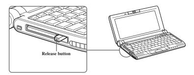
Do not force a card into the slot. It may damage the connector pins.
