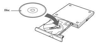
3 Close the tray by pushing it gently. The BUSY indicator on the drive flashes while your computer is reading data from the disc.
