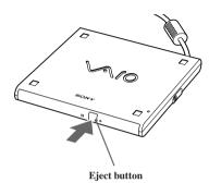
2 Place the disc in the tray with the label side facing up. Push the disc onto the hub until the disc clicks into place.
