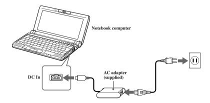
Use your notebook only with the supplied AC adapter. To disconnect your notebook completely from the main power source, unplug the AC adapter. Make sure that the electrical outlet is easily accessible.
