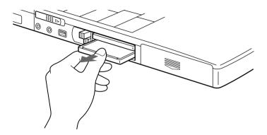
Insert the PC card into the PC card slot, front label facing up. Gently push the card into the slot until the card is fixed into the connector. The release button comes out.
