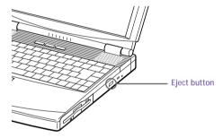
Place a DVD-ROM/CD-ROM in the tray with the label side facing up. For DVD-ROMs, which can be played on both sides, the side of the disc facing up is the side that plays. Push the disc onto the hub until the disc clicks into place.
