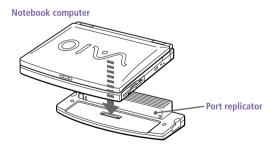
Plug the cable attached to the AC adapter into the DC IN connector on the port replicator. Plug the power cord into the AC adapter and an AC outlet.
