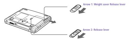
After removing the weight saver, pull out the weight saver's hinged arm and fold it into the weight saver.
