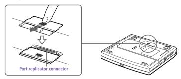
Attach the bottom of the computer to the port replicator connector until it clicks.
