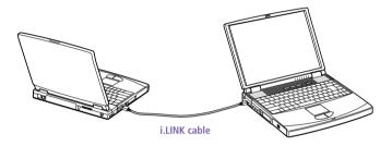
i.LINK cables compatible with your VAIO notebook computer include cables with the following part numbers: VMC-IL4415 (a 1.5-meter cable with a 4-pin connector at each end), VMC-IL4435 (a 3.5-meter cable with a 4-pin connector at each end), VMC-IL4615 (a 1.5 meter-cable with a 4-pin connector at one end and a 6-pin connector at the other), and VMC-IL4635 (a 3.5-meter cable with a 4-pin connector at one end and a 6-pin connector at the other).
