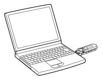
Remove the USB cap and connect the USB connector to a USB connector on your computer. When the remaining battery indication of the display shows: **Full**, charging is completed (charging time is approx. 70 minutes).
