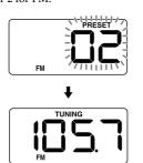
The display shows the frequency for about 10 seconds, and then returns to the current time
