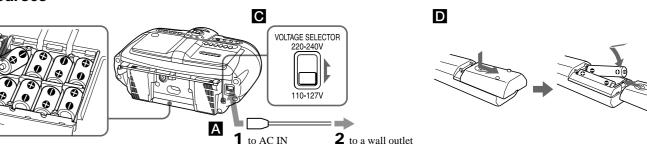
Connect the mains lead A or insert eight R20 (size D) batteries (not supplied) into the battery
