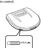
Slide HOLD in the direction of the arrow When you press any button, "Hal d" appears in the display and you cannot operate the player.
