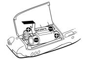
**3** Connect the AC power adaptor. The display and the buttons on the main unit light up for about one minute then go out. The indication "CHG" then appears in the display and charging starts. Charge for about 2 hours (for BP-DM10) or 3 hours (for BP-DM20). (If the battery has been fully charged, "CHG" and flash.)
