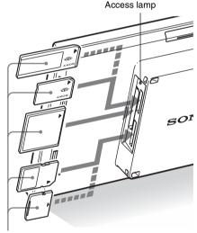
Insert a memory card firmly into the corresponding slot with its label side facing toward you. The slot order from the top is "Memory Stick" ("Memory Stick Duo"), CompactFlash card, SD memory card and xD-Picture Card.
