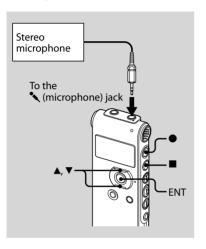
1 Connect an external microphone to the \(^\) (microphone) jack when the IC recorder is in the stop mode.
