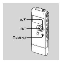
You can select the recording mode in the menu when the IC recorder is stopped. The recording mode is set to "ST" when you purchase the IC recorder.
