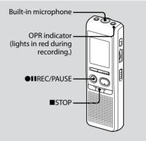
You can record up to 99 messages in each of the four folders (A, B, C, and D). Since a newly recorded message is automatically added behind the last recorded message, you can start recording quickly without searching for the end of the last recording.
