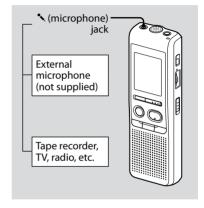
1 Connect a plug-in-power type microphone or other equipment to the \*(microphone) jack.
