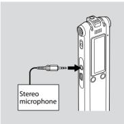
1 Connect an external microphone to the **\*** (microphone) jack when the IC recorder is in the stop mode.
