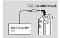
To record the sound of the IC recorder with other equipment, connect the  $\Omega$  (headphone) jack of the IC recorder to the audio input connector (minijack, stereo) of other equipment using an audio connecting cable\*.
