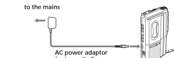
Connect the AC power adaptor to DC IN 3V and to the mains. Use the AC-E30HG AC power adaptor (not supplied). Do not use any other AC power adaptor.
