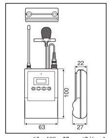
$63 \times 100 \times 27 \text{ mm } (2^{-1}/2 \times 4 \times 1^{-1}/8 \text{ inches}) (\text{w/h/d})$ (excluding the antennas)
