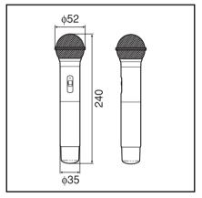
$\begin{array}{c} \phi \ 52 \times 240 \ mm \ (2^{1}/8 \times 9^{1}/2 \\ \text{inches}) \ (\text{dia/length}) \\ \text{Mass} \qquad \text{Approx. 300 g (11 oz)} \\ \text{including batteries} \end{array}$
