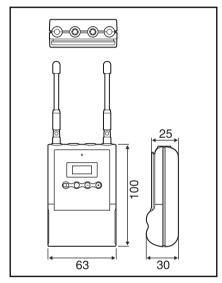
$63 \times 100 \times 30 \text{ mm } (2^{-1}/2 \times 4 \times 1^{-3}/16 \text{ inches}) (\text{w/h/d})$  (excluding the antennas)
