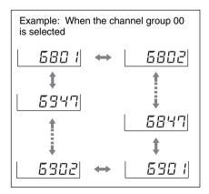
When the desired channel number appears, leave the tuner for about 10 seconds until the selected channel number stops flashing and the selection is stored in memory.
