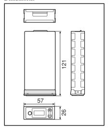
$57 \times 26 \times 121 \text{ mm } (2^{-1}/4 \times 1^{-1}/16 \times 4^{-7}/8 \text{ inches}) (\text{w/h/d})$
