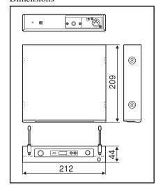
$212 \times 44 \times 209$  mm (8  $^{3}$ /<sub>8</sub> × 1  $^{3}$ /<sub>4</sub> × 8  $^{1}$ /<sub>4</sub> inches) (w/h/d) (excluding the antennas)
