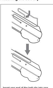
Insert one end of the belt clip into one of two holes on either side of the transmitter, and then insert the other end into the hole on the other side.
