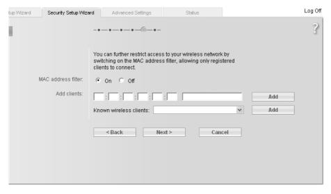
The default setting for access control is disabled. This means that all PCs that use the correct SSID and the right encryption method can log in.
