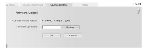
The version of the firmware currently running on your device is displayed in the line *Current firmware version*.
