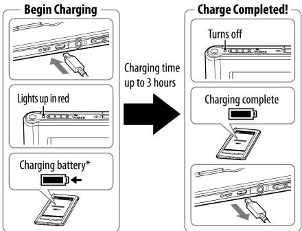
\* The screen will appear after about 5 minutes if charging starts with a completely depleted battery.
