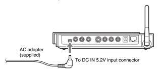
2 Connect the power cord to the AC adapter, and plug it into an AC outlet.
