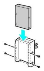
9. Secure the drive to the drive holder with screws, using the two holes on each side of the drive holder.
