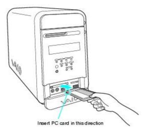
2. If the PC Card does not insert easily, remove it from the PC card slot and verify that it is not upside-down or backwards. Carefully reinsert the PC card, but do not force it into the slot.
