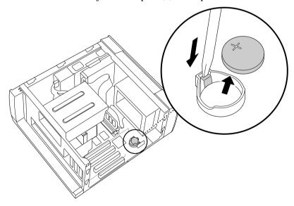
There is danger of explosion if you replace the battery incorrectly. You must replace the battery only with a CR2032 type lithium battery. Discard used batteries according to the instructions on page 80.
