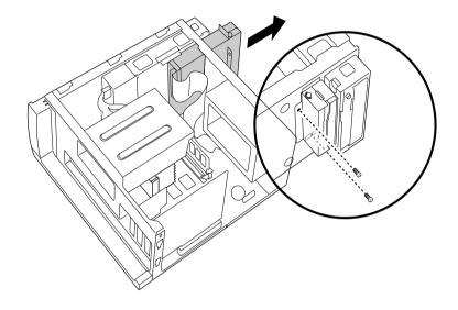
if you are adding memory, you do not need to completely remove the diskette drive or disconnect the cable.
