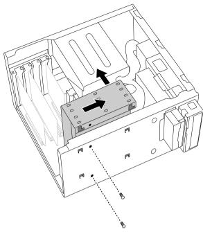
8 Place the drive holder upside down on top of the power supply.
