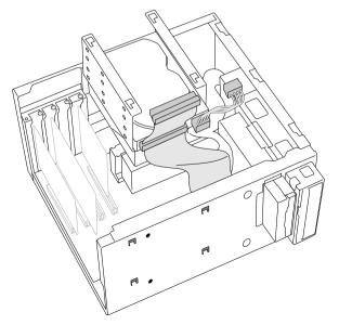
9 Slide the new drive into the drive holder and align the holes on each side of the drive bay.
