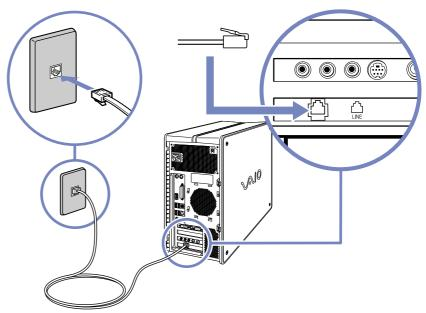
Only DTMF (Dual Tone Multi Frequency) signalling (tone dialling) is supported.
