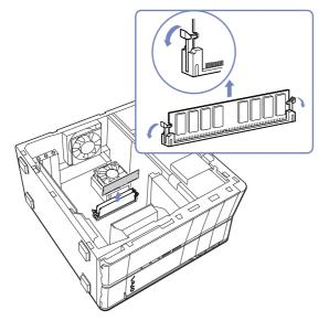
4 To insert a new memory module, remove it from its anti-static package, handling it only by the edges. Download from Www.Somanuals.com. All Manuals Search And Download.
