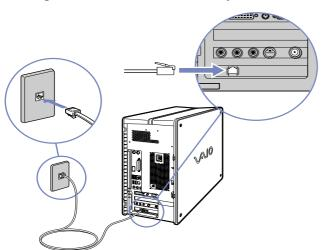
A country-specific phone plug is supplied with your VAIO desktop, allowing you to plug the phone line into the wall jack. We recommend you to use the supplied plug, because the usage of any other phone plug can decrease the connection quality.
