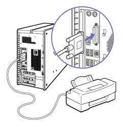
To connect a USB printer, simply plug the printer's USB cable into one of the USB ports on your VAIO desktop. There are USB ports at the front and at the back of your computer.
