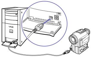
✓ On Sony digital video cameras, connectors labelled DV Out, DV In/Out or i.LINK<sup>™</sup> are i.LINK<sup>™</sup>-compatible.
