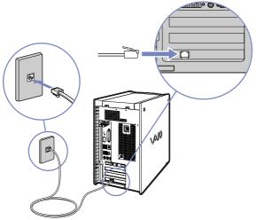
A country-specific phone plug is supplied with your VAIO desktop, allowing you to plug the phone line into the wall jack. We recommend you to use the supplied plug, because the usage of any other phone plug can decrease the connection quality.
