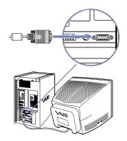
in There are two ports: one for DVI screens and one for common VGA and CRT screens. Make sure you are using the appropriate connector.
