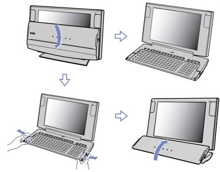
With the **Keyboard Closure Setup** software installed on your computer, your computer launches an appropriate software application when you shift the keyboard from one position to the other. Download from Www.Somanuals.com. All Manuals Search And Download.
