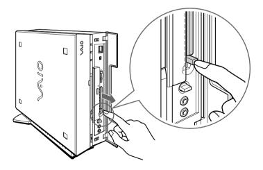
The card is ejected from the card connector. Remove the card by holding it by its edge and pulling it out carefully.
