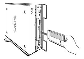
When the card is completely inserted, the eject button pops out.if you cannot insert the card, do not forcibly insert it. In this case, make sure the card is not inserted upside-down or backward, and then reinsert the card into the slot carefully.
