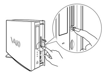
When the PC card is ejected from the card connector, remove the card by holding the edges and pulling it out carefully.
