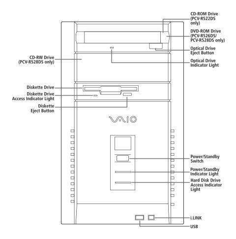
For your convenience, your computer includes USB and i.LINK connectors on both the front and back panels, allowing you to connect to either set of connectors. The i.LINK connector on the front of your system is a 4-pin connector.
