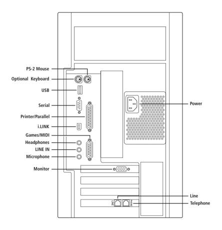
For your convenience, your computer includes USB and i.LINK connectors on both the front and back panels, allowing you to connect to either set of connectors. The i.LINK connector on the back of your system is a 6-pin connector.
