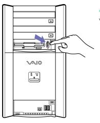
Always remove the Memory Stick<sup>TM</sup> gently, or it may pop out unexpectedly. You are recommended to remove the Memory Stick<sup>TM</sup> before shutting down the computer.
