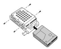
Secure the drive to the drive holder using screws in each of the two holes on each side of the drive holder (screws are provided with the new drive). Do not overtighten the screws.
