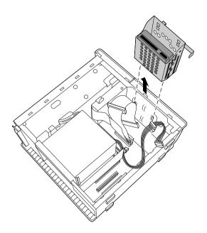
7 Slide the new drive into the bottom part of the drive holder and align the holes on each side of the drive holder.
