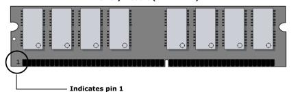
Align pin 1 of the Dual Inline Memory Module (DDR-DIMM) to the small triangle located on the memory module slot of the system board.
