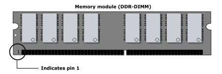
7 Carefully but firmly insert the edge of the module into the socket.
