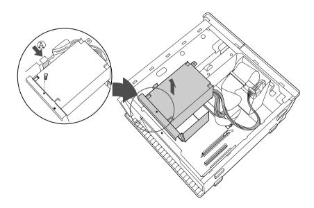
4 Rotate the power supply upside down and rest it on top of the chassis where the hard drive is located.
