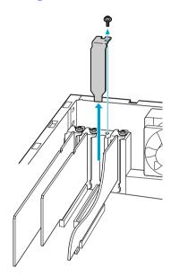
☐ Install the add-on card by inserting it into the expansion slot and secure it with the screw from the expansion slot cover.
