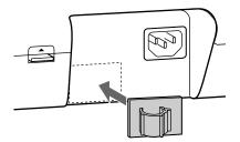
**3** Plug the power cord into the AC input port on the back panel of the computer.
