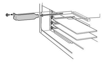
5. Install the add-on card by inserting it into the expansion slot and securing it with the screw from the expansion slot cover.
