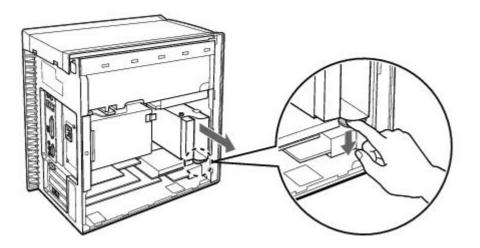
7. Slide the new drive into the drive holder and align the holes on each side of the drive bay.
